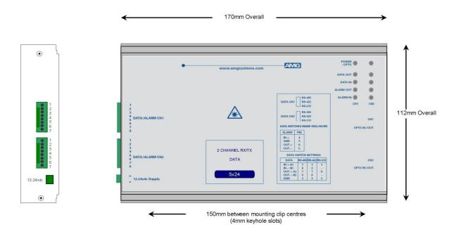
The **AMG5524** is a **DUAL** standalone system which provides two independent channels, each designed to transmit and receive one bi-directional alarm plus one data signal over one Singlemode optical fibre.
